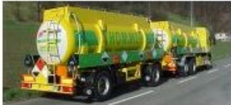
Tanker train for chemicals (40 tonnes)
