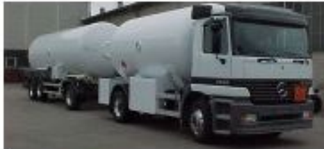
Tanker train for liquid gas (40 tonnes)
